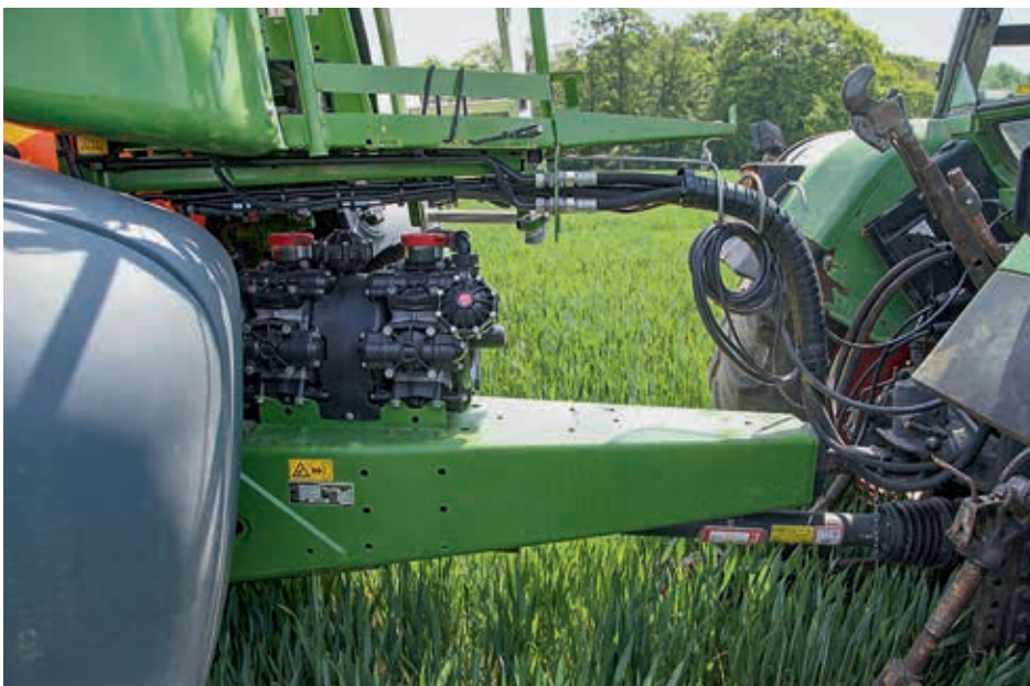
Test machine spec included a top-mounted drawbar and pto/belt driven pump. The load-sensing system with accumulator charging function was an interesting feature.
