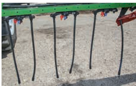
The nozzle holders with extension kit for 25cm spacings are controlled individually and can be fitted with drag hoses.
