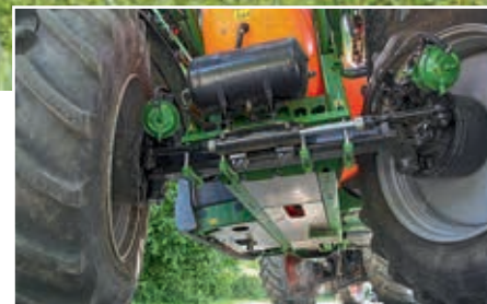
A 2.25m track-width offers enough room for 520/85 R42 rubber and 26° turns. Ground clearance is 0.80m.
