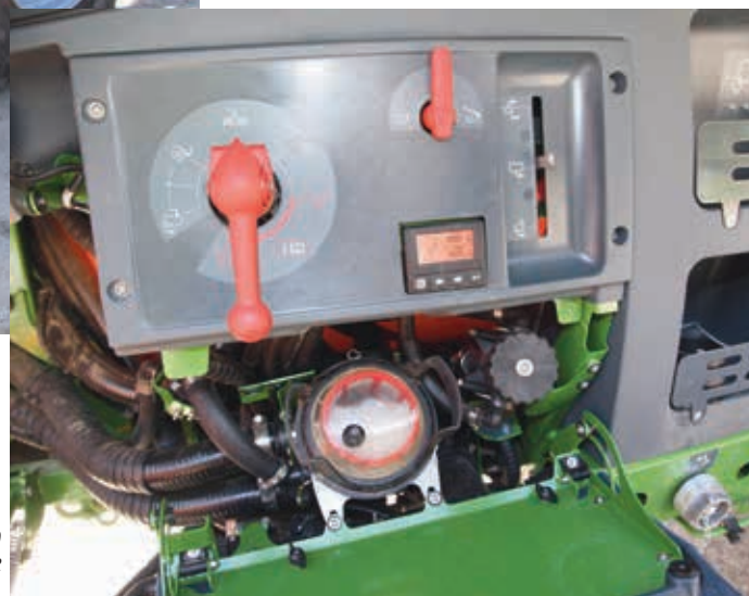
The Comfort Pack buys an electric suction tap with neighbouring LCD Display. The selector valve on the pressure side is still operated manually.
