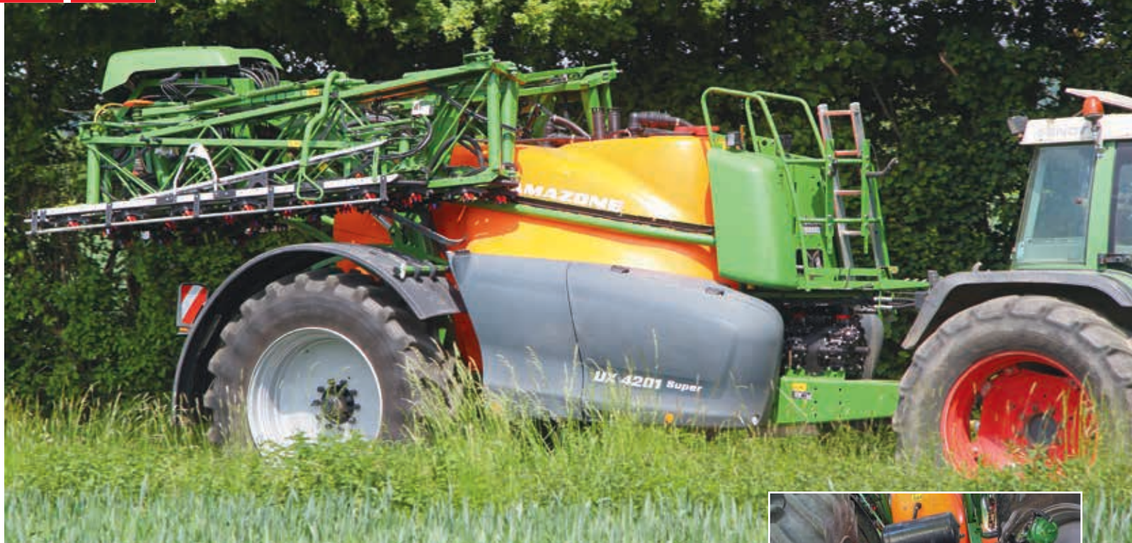
The Super L boom swiftly folds into a compact package. Load-sensing brakes and a 12.5t gross weight allow you to travel at 60km/hr even when filled with ammonium nitrate urea solution.
