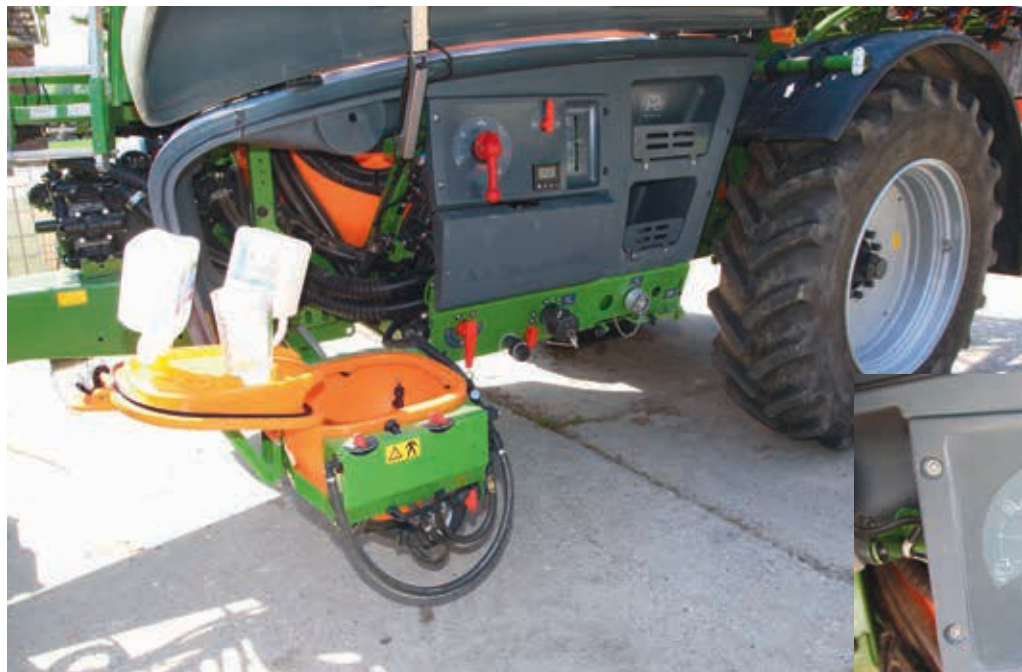
The induction hopper has an astounding suction rate. If specified with a double-pump and injector, this rate is a whopping 705l/min.
