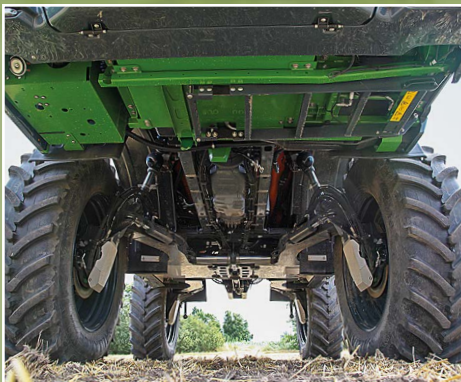
The chassis with independent suspension is new; the hydraulic track width adjustment of up to 75cm is standard. Another trick is the ground-friendly ability to offset the front and rear wheels.
