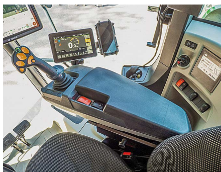
The new Claas-sourced cab is spacious and now has an Amazone-developed armrest.
