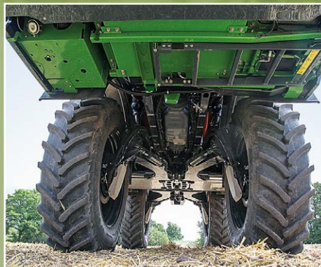
The chassis with independent suspension is new; the hydraulic track width adjustment of up to 75cm is standard. Another trick is the ground-friendly ability to offset the front and rear wheels.
