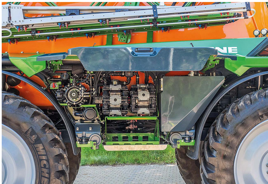
The Comet pumps are located to the right of the tank and deliver 260 + 350l/min.
