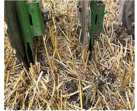
Michael Seelmeyer can sow legumes via an additional coulters bank which runs behind the seed coulters discs.
