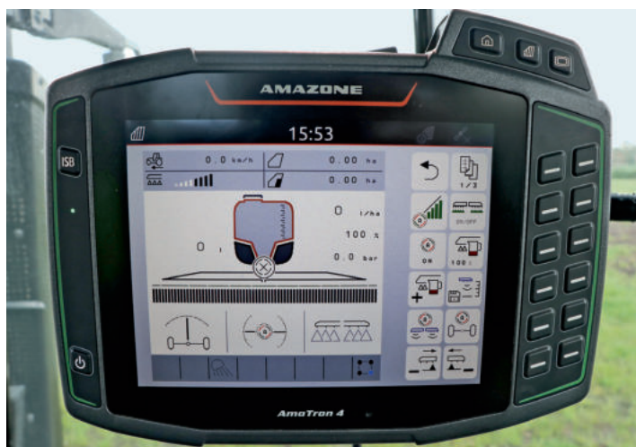
At the heart of every sprayer is an ISOBUS-compatible terminal which controls the application rate and switches boom sections and nozzles.
