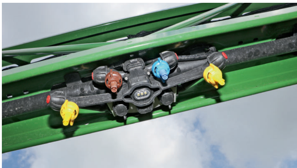
The AmaSelect kit spaces the yellow nozzles 25cm apart and all nozzles have LED's.
