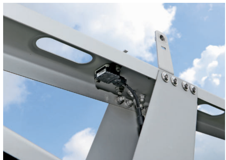
Acceleration sensors on the boom ends measure the speed for SwingStop and CurveControl.
