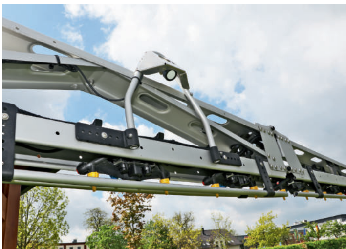
Ultrasonic sensors monitor the boom-to-target distance and the hydraulic rams follow suit adapting the boom height.
